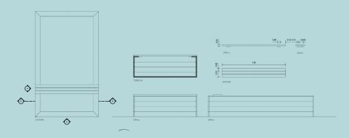
Dimensions: Individual Module Width: 2500mm Length: 1500mm Height: 400mm
